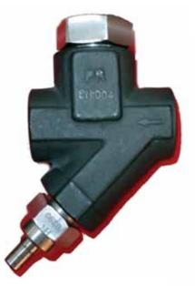
**Ratings** Design: 600 psig, 750°F Operating: 4 to 450 psig/750°F [0.3 to 31 bar/400°C] **711HP/721HP only** Design: 650 psig, 750°F Operating: 150 to 650 psig/750°F [10.3 to 45 Bar/400°C] Applicable Codes and Standards End connections per ANSI B1.20.1 for threaded ends, per
